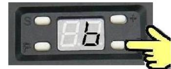
The display shows a "0" for disabled, or "1" for enabled. Use + and - buttons to select.
