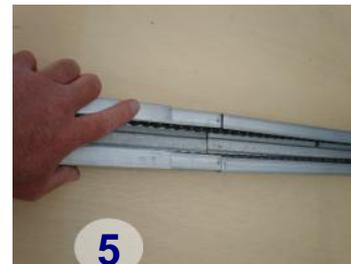
Slide the locking sleeves across the rail ends. This is not easy. It best done on a flat surface. If continues to resist, check the ends of the rails for damage.
