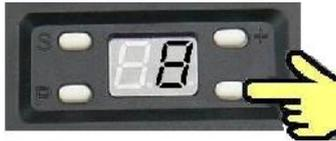
The display shows a flashing channel number (from 1 to 4). Use the + and - buttons to select a channel number.
