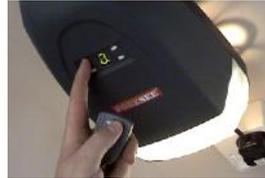
To start, press and hold "P" for 5 seconds. The display shows step 1.
