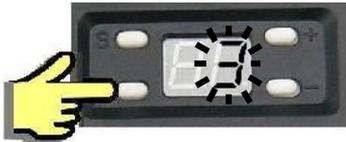
Press “P” to run a closing test. When the door is closed fully, press “P” to save.
