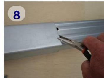
When the sections are joined together, turn the rail over, then turn up all the remaining locking tabs.
