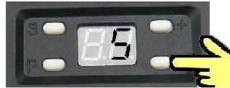
The display shows a flashing “5” and the door rises. Block the beam. “A” should be displayed. If not, check wiring.
