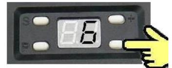
Use + and – keys to select step 6 then press “P” to display the force setting character. Adjust with + and – keys. Press “P” to save.
