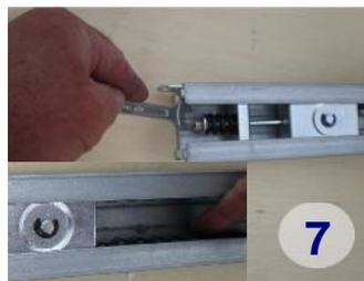
Tighten the chain checking for tension. The chain should move sideways, but not touch the top or bottom of the rail
