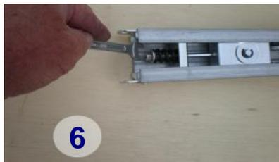
Check that the chain engages properly with both cog wheels. The chain should be long enough. Slacken off the spring if necessary
