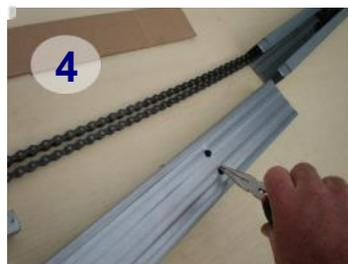
Turn over the centre rail section and turn up the four locking tabs.
