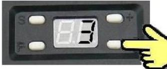
Press “P” to start the test. The 3 flashes as the door opens. When it has stopped, press “P” to save the force settings.
