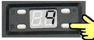
Use + and - keys to select a delay as required, then press "P" to save.
